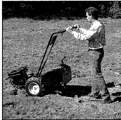
Figure 4-4: To begin turn, reduce engine speed and lift handlebars until engine and tines are balanced over wheels.
